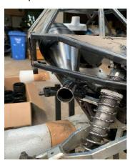
You will have to shorten the Front Right (ex side) body cage pin to make sure it doesn't hit the pipe. We have just left you enough room to get the pipe through and get a clip into the closest pin hole. The cut off all extra length beyond this pin hole.
