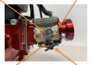
Low Speed mixture adjustment screw Base setting:- 1 3/8 turns out
