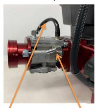
Pulse feed pipe (do not remove)
