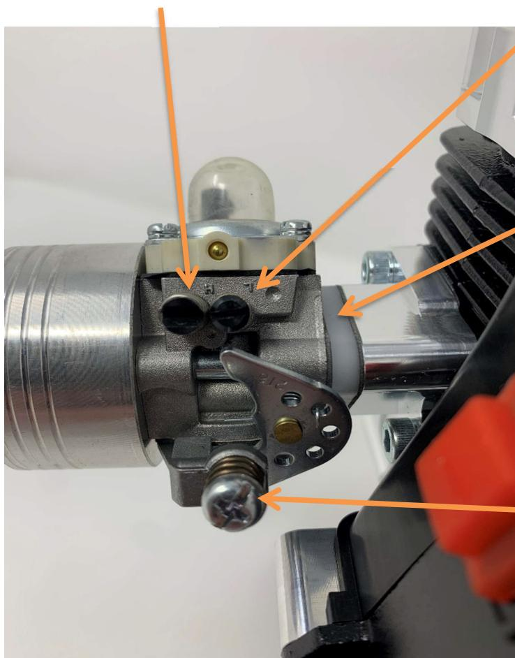
Heat isolator with high temp gasket
