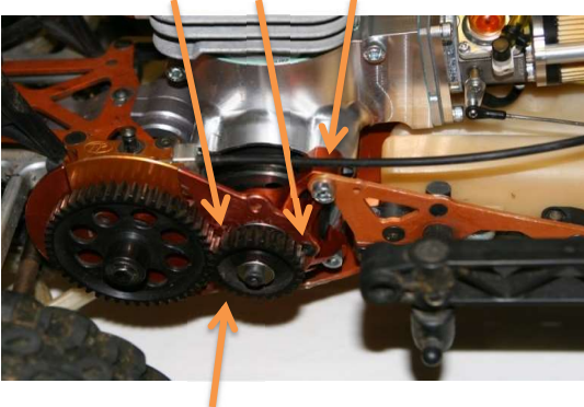
Right side mounting bolts (2 behind pinion)
