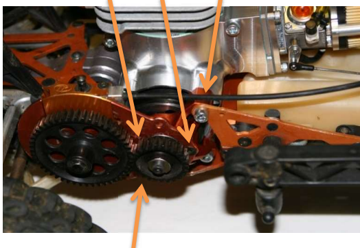
Right side mounting bolts (2 behind pinion)
